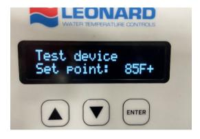
This Error indicates that it is time to test the valve, per ANSI Z 358.1. This message will automatically display once every 7 days to remind facility personnel to run emergency fixtures to ensure all components of the emergency water system is properly functioning. This error has no effect to the valve's operation and can be cleared by pressing the ENTER button.
