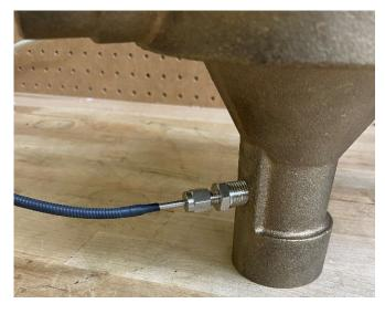
INSTALLATION OF COMPRESSION FITTING AND OUTLET RTD PROBE ON NEUTRON VALVE BODY
