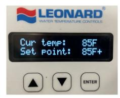
The user is returned to the 'Home Screen' which displays current temperature as measured on valve outlet and the set point temperature on the line below.
