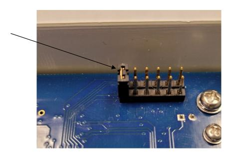
If the jumper is installed in the first slot the unit will display in degrees "F", with the jumper removed the unit will display in degrees "C". If the unit is ordered as a degree "C" unit the jumper will be removed at the factory and shipped loose in case the customer would like to switch it back to degree "F".
