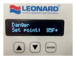
This Error indicates that the outlet temperature leaving the valve is outside of the tepid water temperature range, 65-95°F. The message will alternate with the Current Outlet Temperature.
