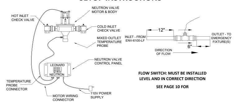
The Neutron Control Box has a 2 Line, 16 character LED digital display screen, which serves as the User Interface by utilizing a simple 3-button keypad interface:  $\blacktriangle$ ,  $\blacktriangledown$  and ENTER, to change temperature see page 4.
