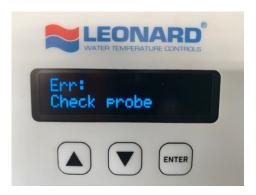
This Error indicates that the RTD Temperature Probe installed in the valve outlet is either disconnected from the Control Box or the wires are broken and it is in need of replacement. Please verify 3 wire connector on left side of control box is firmly engaged and verify that wires are continuous to the probe end. Replace if necessary. See Page 10 for details.
