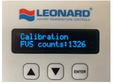
The above Calibration Screen is used to enter the initial Full Valve Sweep Value obtained and recorded in Step #10 from initial power up. Press **ENTER** to input FVS value, it will flash. Use ▲ button to adjust FVS counts value and advance until it agrees with the Initial Sweep Value recorded in Step #10 above. Press **ENTER** to save the FVS counts value. To Exit Calibration: Press the ▲ ▼ buttons simultaneously. This will return you to the HOME Screen:
